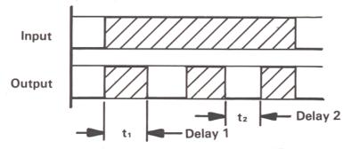
Delay 1 = "on" time Delay 2 = "off" time
