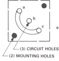
a & c must be interconnected in the circuit module
